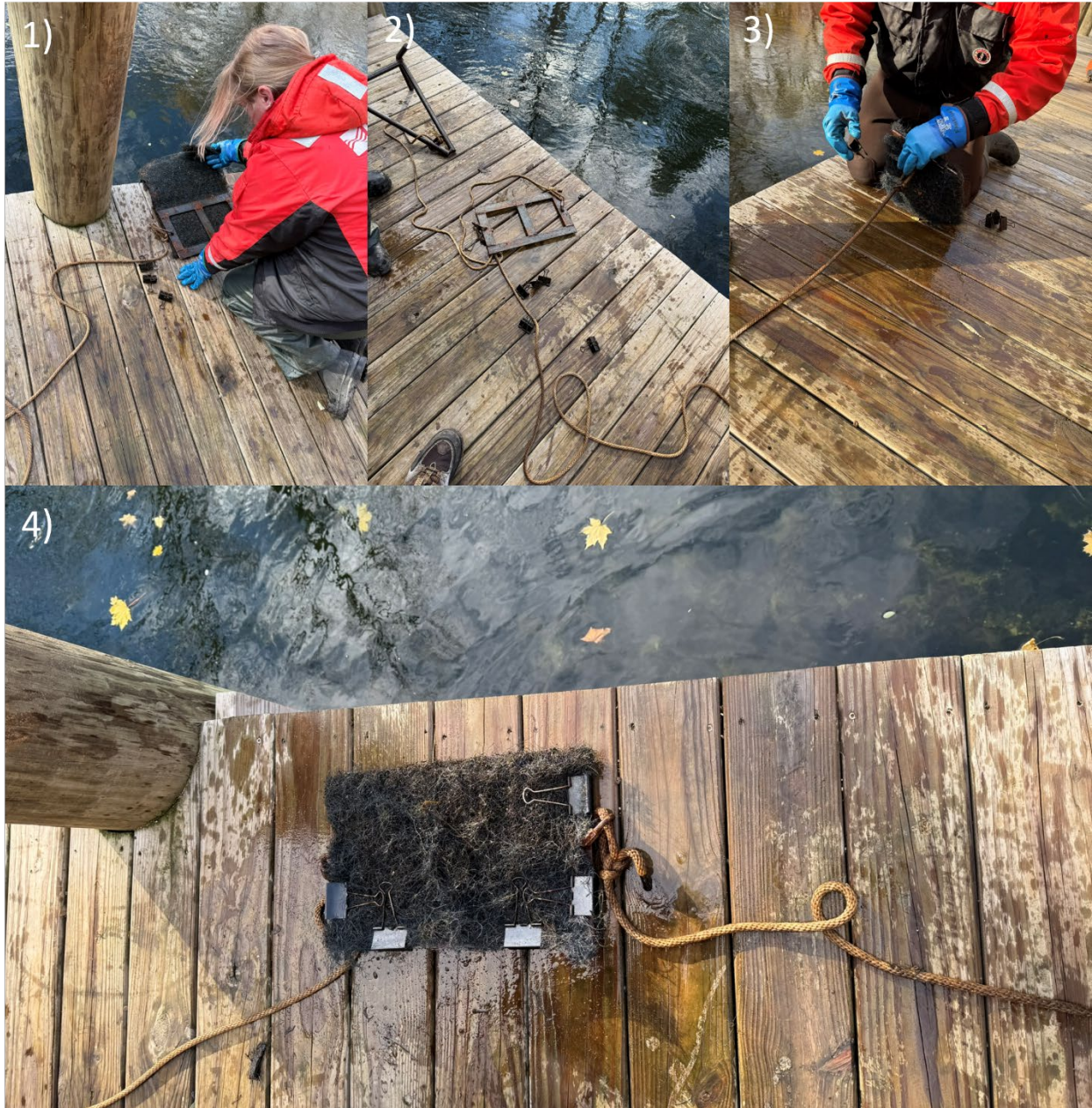
Figure 2. Staff from the U.S. Geological Survey (USGS) processing an egg mat chain in the Boardman/Ottaway River on 22 November 2024. (1) inspection; (2) disassembled egg mat frame; (3) reassembly of an egg mat; and (4) a single mat prior to deployment. Egg mats are used to sample fertilized and drifting eggs in the river.
